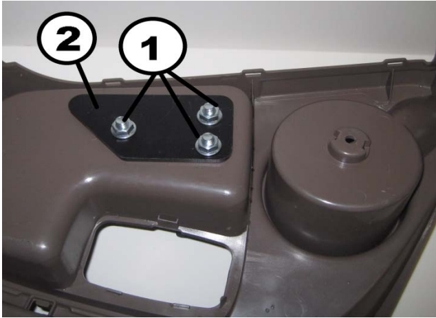
Figure 6. Installation of Backing Plate Key 1 – 5/16” Flange Nut Key 2 – Backing Plate – Note orientation
