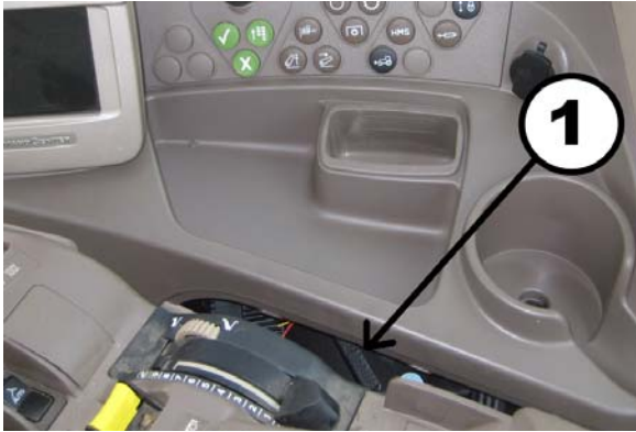
Figure 2. Access Panel Removal Key 1 – Access Panel
