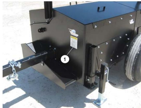
Figure 2. Safety Sign Location Key 1 - Safety Sign
