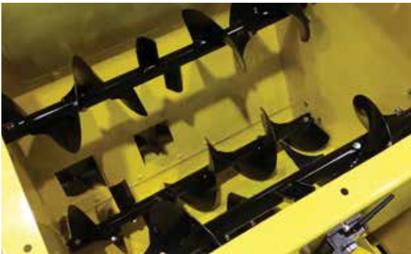
Lower sample hopper provides for mixed samples and even feeding to discharge system through the use of three augers, handling even the most demanding crops.
