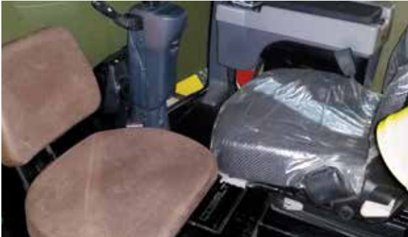
Assistant seat in the air-conditioned cab reduces fatigue in sample collection. Operator can also collect samples if assistant is not available.
