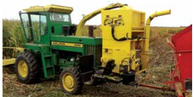
The RCI 130S Research Plot Sampler mounted to a John Deere 5400 Series Self-Propelled Forage Harvester
