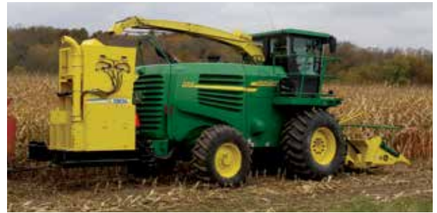
The RCI 130S Research Plot Sampler mounted to a John Deere 7300 Series Self-Propelled Forage Harvester
