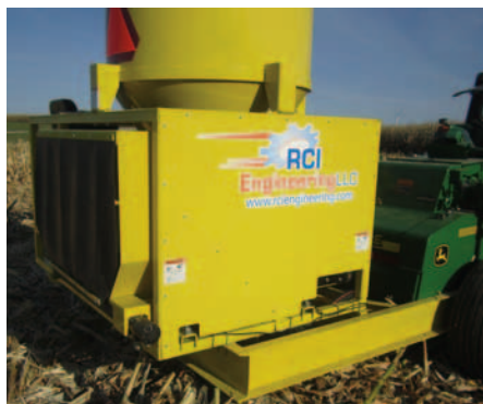
The RCI 30A mounts to the John Deere pull-type or self-propelled forage harvester in about 4 hours.
