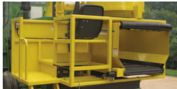
Harvest samples with or without an operator on the 30A unit. The operator station allows immediate sub-sampling of the harvested crops.
