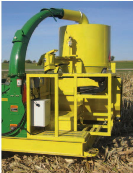
Harvest samples with or without an operator on the 30A unit. The operator station allows immediate sub-sampling of the harvested crops.
