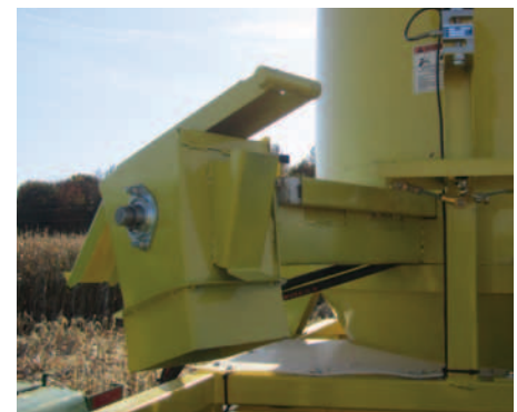
Sub-sampling is an easy task. The cross auger pulls material from the drum, weighs and stores it.
