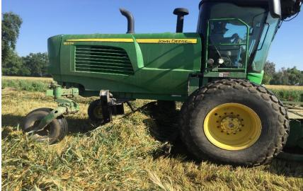
The R1 Merger Attachment is available for the John Deere W200-Series (W235/W260/W200M/W235M/W235R/W260R) Self Propelled Windrowers (SPW) with 500R/R500 Rotary Platforms. The R1 allows merging of windrows with SPW in front of a self-propelled forage harvester, or in conditions that do not require wide swaths for dry-down. The R1 can eliminate the need for raking or merging passes through the field.
