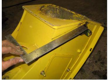
6/ Weld RC0133 Bottom Plate onto the spout as shown in red below (Item A). Weld around the perimeter of the new part to match the opposite side.
