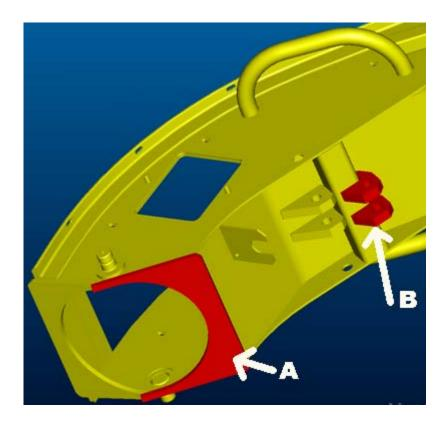
7/ Weld RC0132 ears for lift cylinder to the spout cross tube as shown above (Item B). Weld the ear to the cross tube on both sides of each ear, making sure to align the inside edges with the existing ears so the hydraulic cylinder will fit into the opening.
