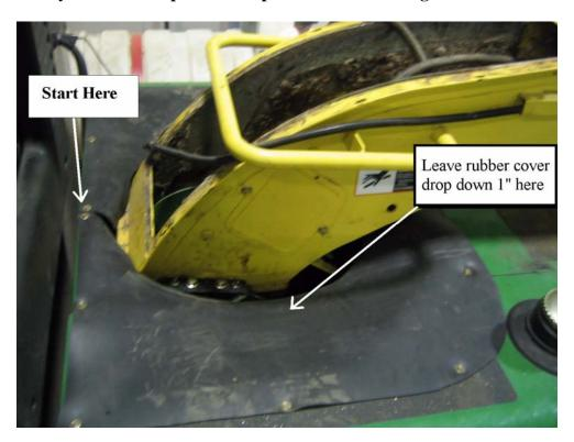
Note: Install "DO NOT STEP" and "RCI" Decals as shown below on each rubber cover. Always install covers with decal showing on top of machine.
