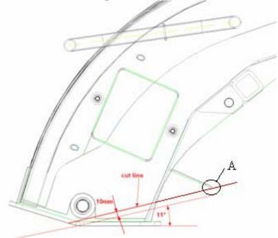
Note: It is easies to make the cut by tracing a line that is flush with the boss of the pivot pin at the center, and extend it to the rear face of the spout using a straight edge. Align the straight edge with the bracket used to hold the accumulator in place on the bottom of the spout (shown in location A). See picture below.
