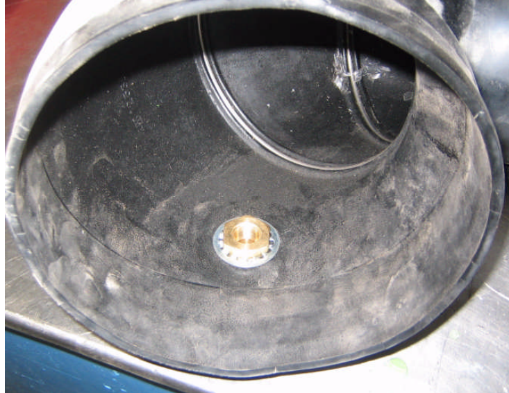
Figure 17. Installation of Bulkhead Connector Fitting
