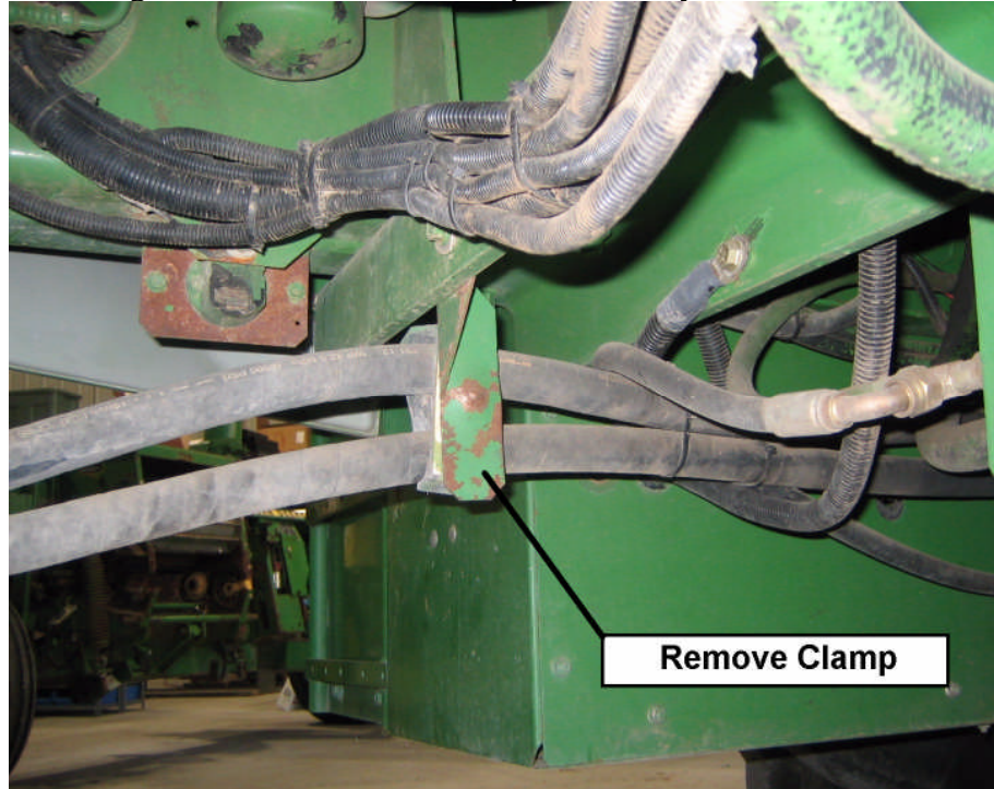
Figure 27. Removal of Clamp on Rear Hydrostatic Hoses
