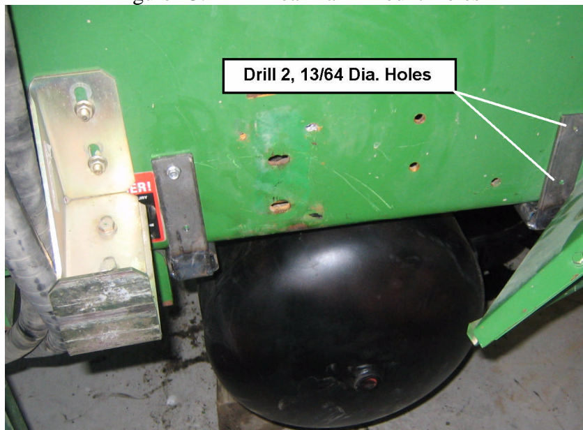
Figure 43. Drill Rear Tank Mount Holes
