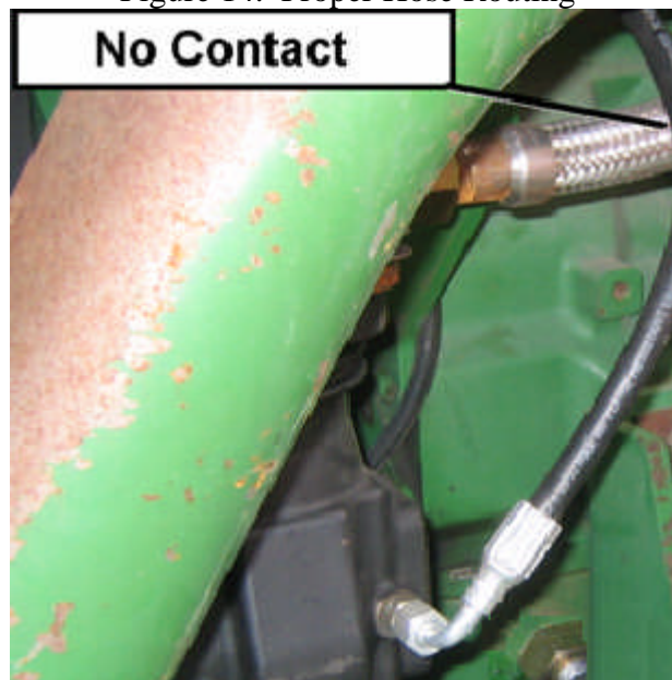
Figure 14. Proper Hose Routing
