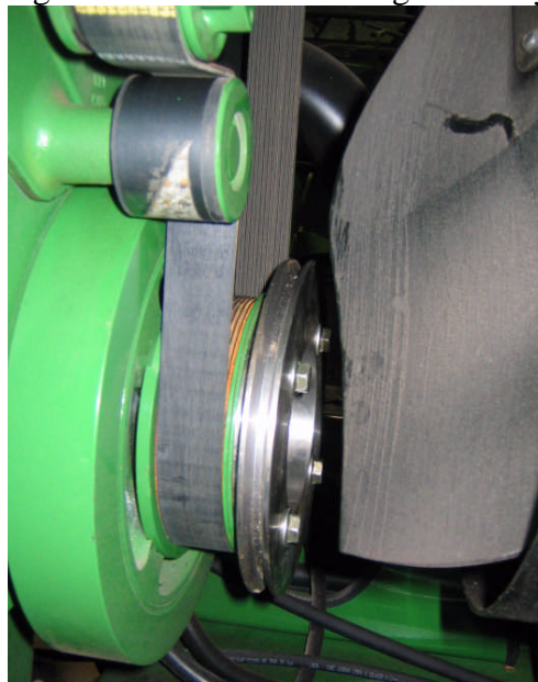
Figure 5. Installation of Engine Pulley
