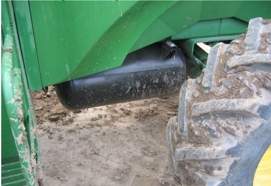
Figure 25. Completed Air Tank Installation
