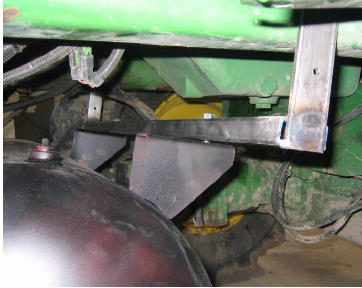
Figure 42. Rear Tank Frame Member for Assembly
