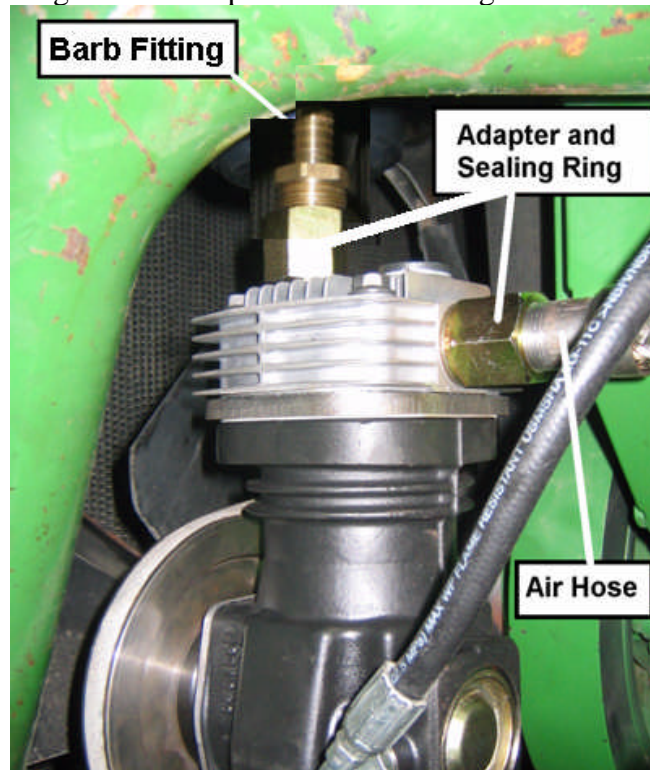
Figure 13. Adapter and Barb Fitting Installation
