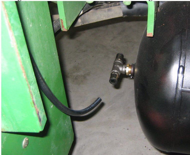
Figure 51. Installation of Air Line to Storage Cabinet
