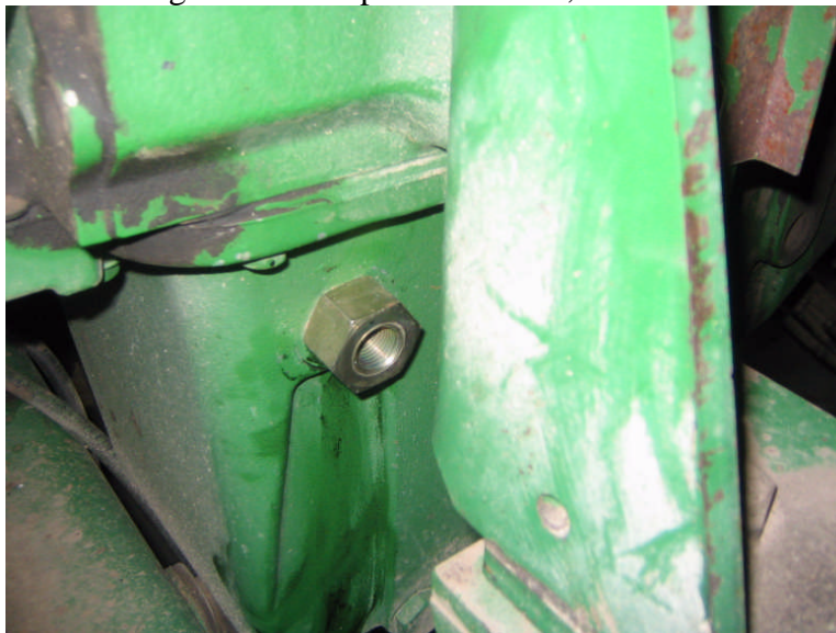
Figure 12. Adapter in Oil Pan, Installed.
