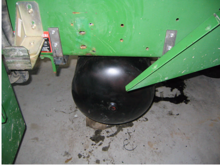
Figure 37. Completed Air Tank Installation, LH Side
