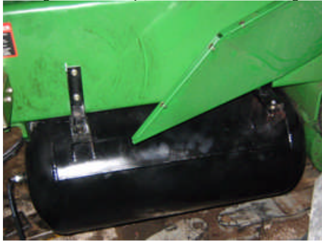
Figure 32. Completed Air Tank Mounting
