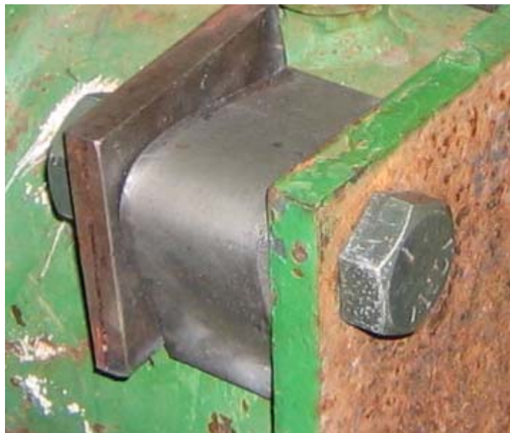
Figure 2. Install bolt to hold flange and gusset in place for welding.
