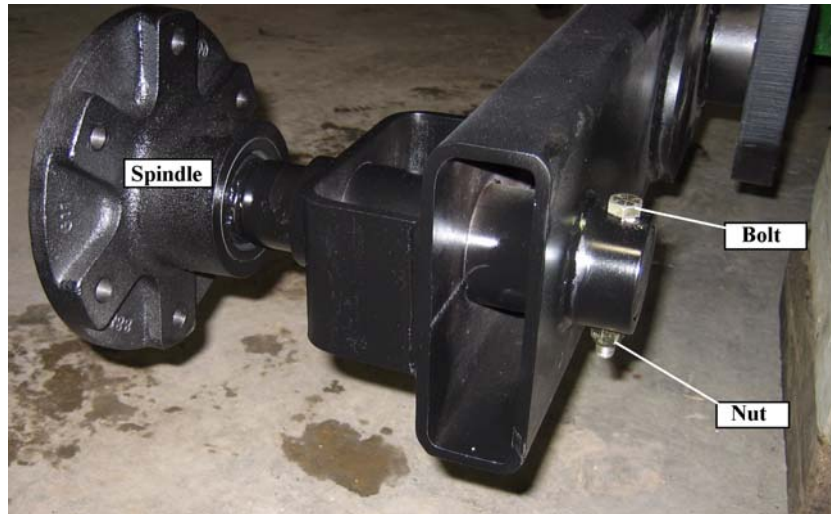
Figure 9. Assembly of Spindle to Walking Beam
