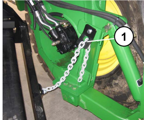
Figure 16. Front Chain Installation
