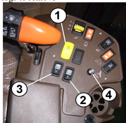
Figure 2. Switches Installed 1 – DWA On/Off 2 – Belt Frame Raise/Lower 3 – Deflector Raise/Lower 4 – Belt Speed Control
