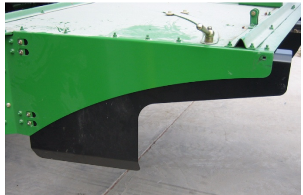
Figure 2. LH Forming Shield End Result
