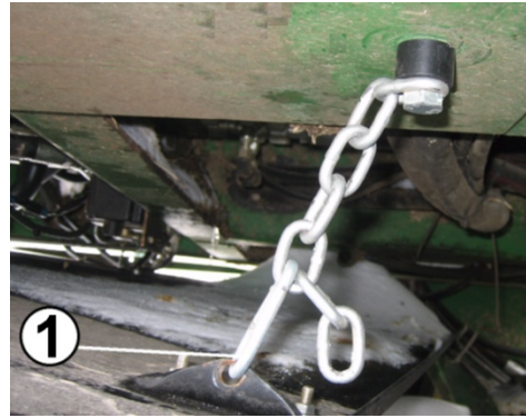
Figure 8. Chain Hook Removal
