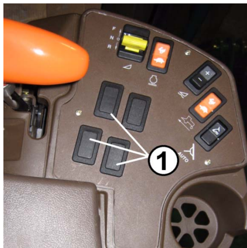
Figure 1. Armrest Plate 1 – Plugs to remove
