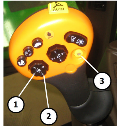
Figure 1. Hydrostatic Control Handle Key 1 – Directional Control Key 2 – Deflector Control Key 3 – WMA Enable / Disable Control
