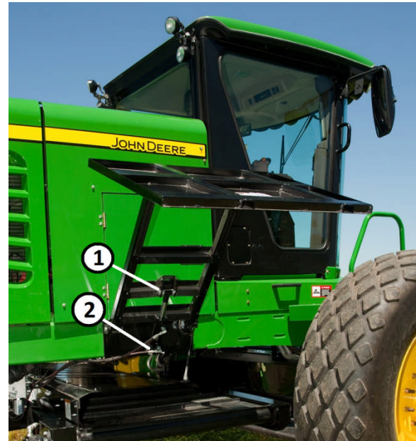
Figure 1. Deflector Cylinder Positions Key 1 – Rod End of Cylinder Key 2 – Base End of Cylinder
