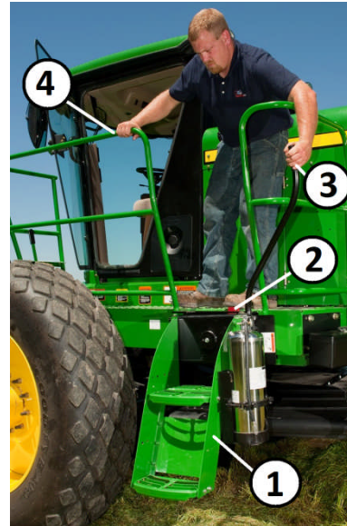
Figure 6. Raising Ladder for LH Discharge
