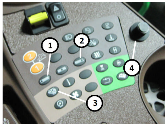
Figure 3. Cross Belt Controls Key 1 – Cross Belt Raise Key 2 – Cross Belt Lower Key 3 – Cross Belt Speed Adjust Key 4 – Adjustment Dial
