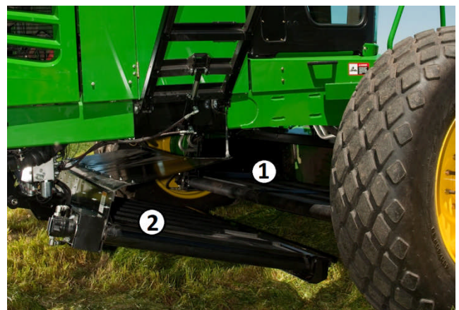
Figure 7. Power Table and Cross Belt Key 1 – Power Table Key 2 – Cross Belt
