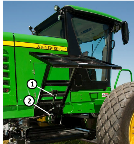
Figure 1. Deflector Positions Key 1 – Rod End Positions Key 2 – Base End Positions
