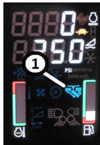
Figure 4. Lower Cornerpost Display Key 1 – Cross Belt Speed Adjust Indicator
