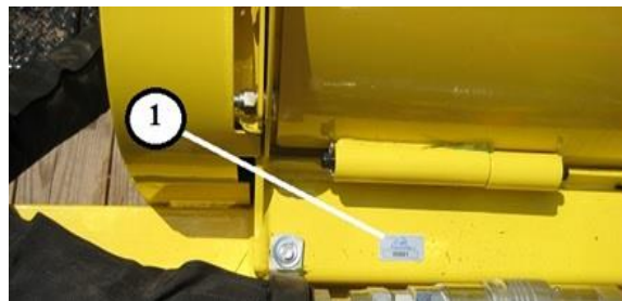
Figure 30. Back of Unit Key 1 – Serial Number Location
