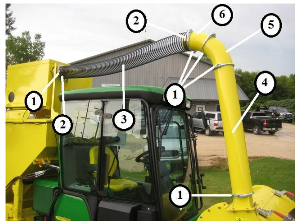
Figure 10. Attaching the discharge pipe Key 1 – Quick Clamp 6" (as required) Key 2 – 6" Hose Clamp Key 3 – Flexible Tubing Key 4 – Discharge Pipe (straight) Key 5 – Discharge Pipe ( 45 degree) Key 6 – Discharge Pipe (30 degree)
