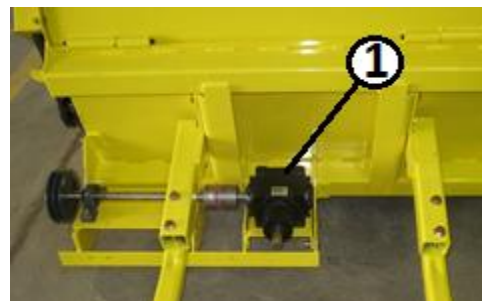
Figure 22. Main Gearbox Key 1 – Fill Hole (breather removed for clarity)
