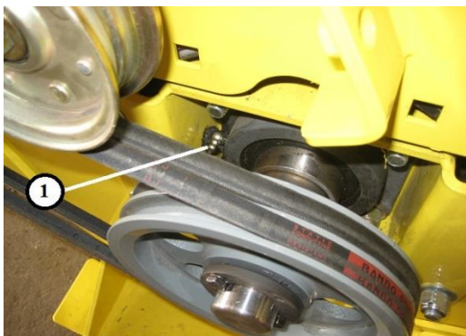
Figure 15. Flail Drive (RH Side of Head) Key 1 – Grease Fitting Location
