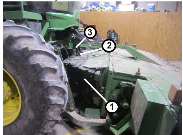
Figure 108. Platform Installation Key 1- Forming Shield Key 2 – Link Mount Key 3 – Forming Shield Link
