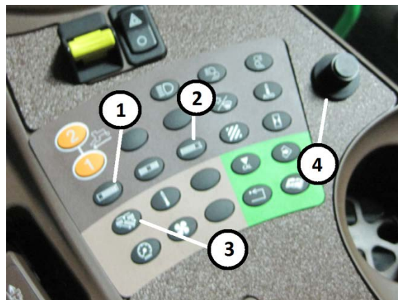
Figure 8. Cross Belt Controls Key 1 – Cross Belt Raise Key 2 – Cross Belt Lower Key 3 – Cross Belt Speed Adjust Key 4 – Adjustment Dial
