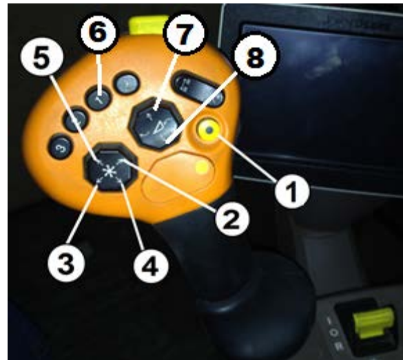
Figure 4. Merger Controls Key 1 – Merger Enable/Disable Key 2 – Belt Speed Increase Key 3 – Belt Speed Decrease Key 4 – Manual Merger Lower Key 5 – Manual Merger Raise
