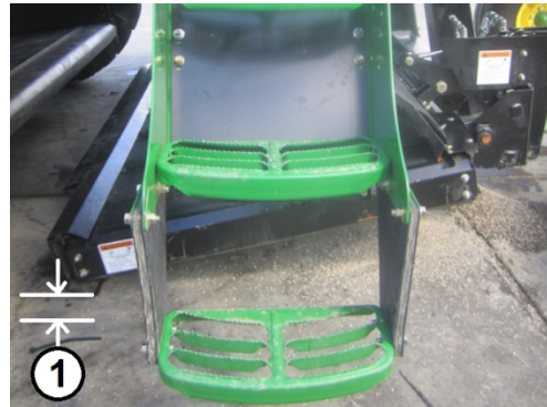
Figure 28. Ground Clearance Measurement Key 1 – Point of Measurement
