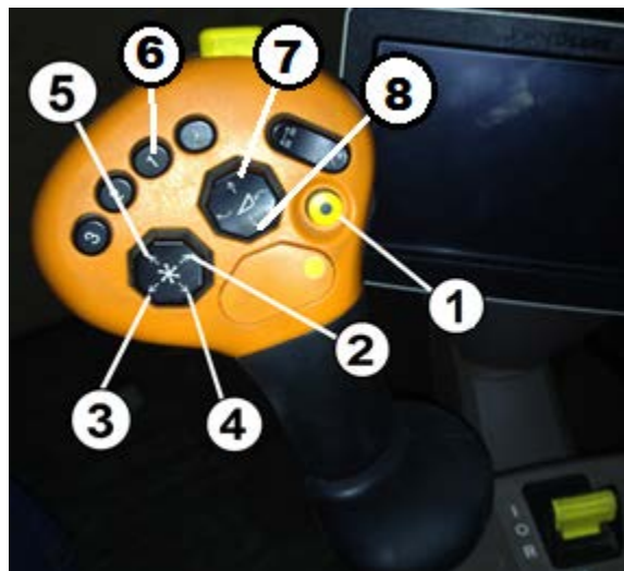
Figure 2. Merger Controls Key 1 – Merger Enable/Disable Key 2 – Belt Speed Increase Key 3 – Belt Speed Decrease Key 4 – Manual Merger Lower Key 5 – Manual Merger Raise Key 6 – “1” Button Key 7 – Platform Raise Key 8 – Platform Lower
