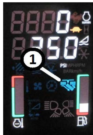
Figure 9. Lower Cornerpost Display Key 1 – Cross Belt Speed Adjust Indicator
