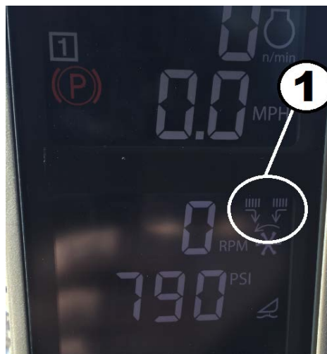
Figure 3. Merger Enable Indicator Key 1 – Merger Enable Icon Illuminated
