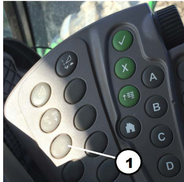
Figure 5. Front Belt Motor Override Key 1 – Front Belt Motor Disable Button
