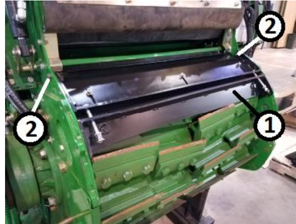
Figure 4. Upper Assembly Installation Key 1 – Upper Assembly Key 2 – Hardware Locations
