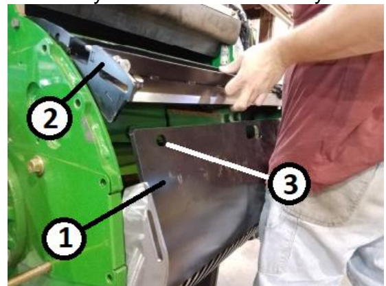
Figure 31. Screen Removal Key 1 – Screen Key 2 – Upper Assembly Key 3 – Alignment Hole
