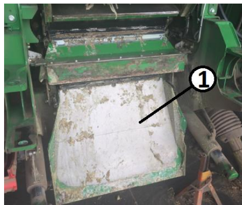
Figure 24. Bottom Pan Lowered (CH Removed for clarity) Key 1 – Pan
