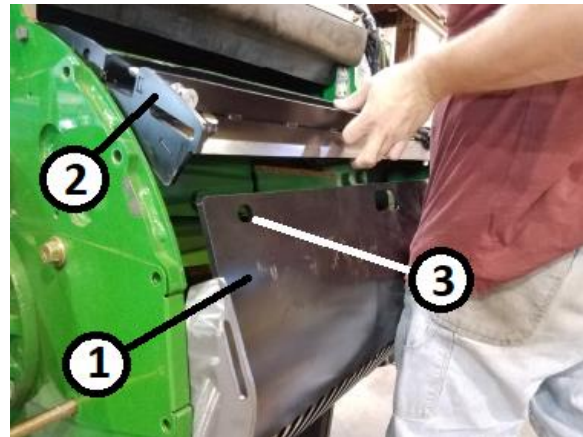
Figure 37. Screen Installation Key 1 – Screen Key 2 – Upper Assembly Key 3 – Alignment Hole
