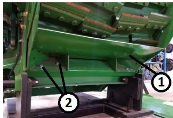
Figure 2. Spiral Band Removal Key 1 – Spiral Band Key 2 - Hardware
