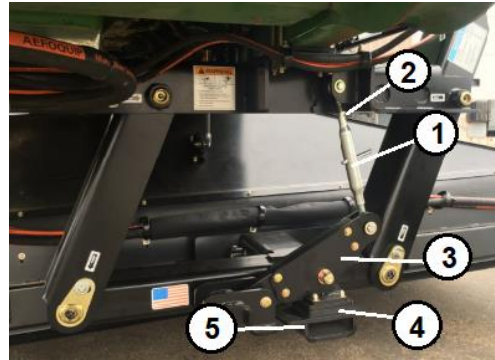
Figure 35. Adjustment Components Key 1 – Linkage Key 2 – Jam Nut Key 3 – Pivot Arm Key 4 – Slider Key 5 – Pivot Frame
