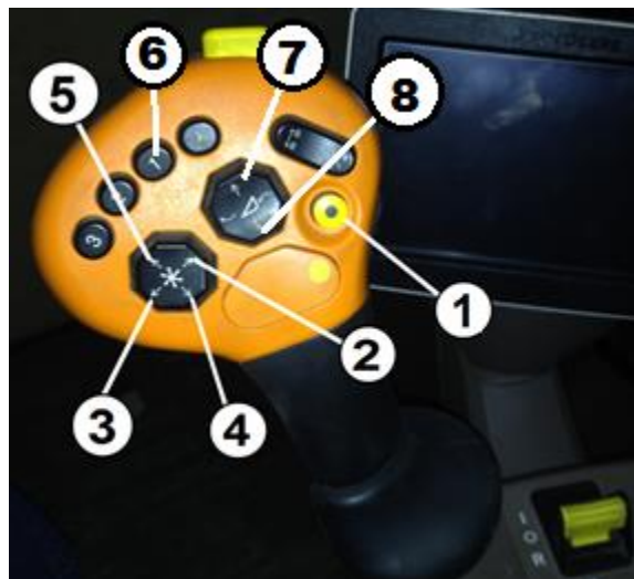
Figure 10. Merger Controls Key 1 – Merger Enable/Disable Key 2 – Belt Speed Increase Key 3 – Belt Speed Decrease Key 4 – Manual Merger Lower Key 5 – Manual Merger Raise Key 6 – “1” Button Key 7 – Platform Raise Key 8 – Platform Lower
