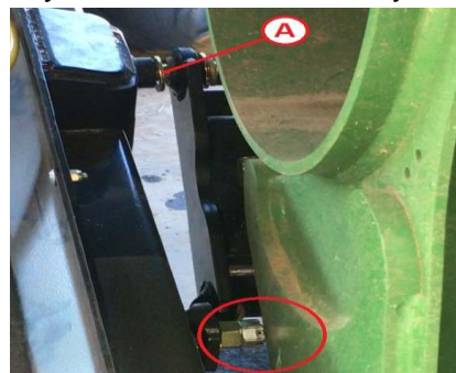
Figure 106. LH Wheel Drop Clearance (View from front look back at LH side)
