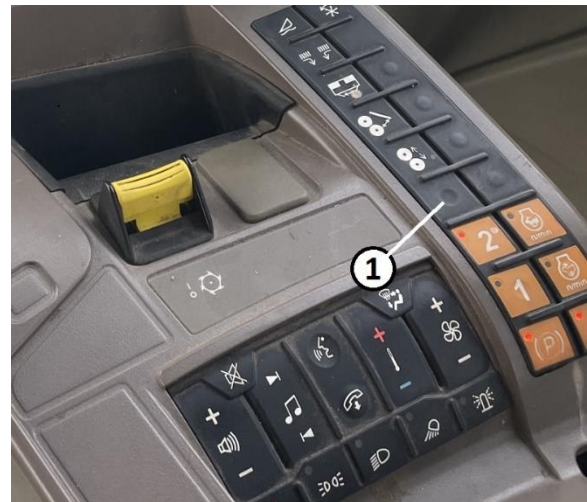
Figure 9. Front Belt Motor Override Key 1 – Front Belt Motor Disable Button
