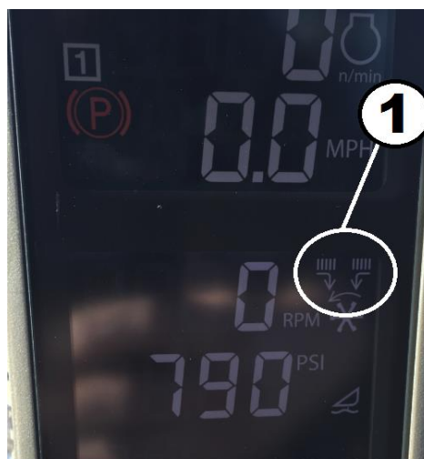
Figure 11. Merger Enable Indicator Key 1 – Merger Enable Icon Illuminated
