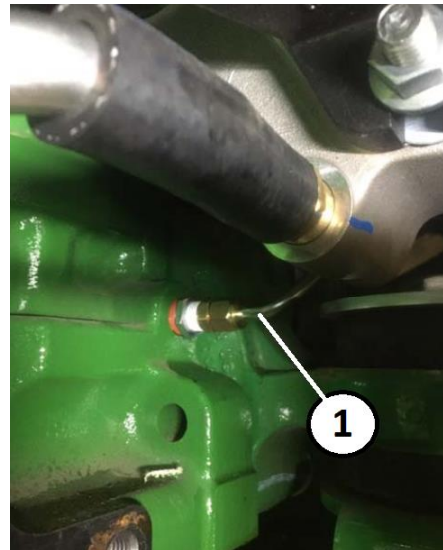
Figure 60. Pressure Port Install Key 1 – Pressure Line
