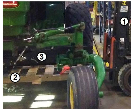
Figure 111. Cross Belt Positioning Key 1 – Forklift Key 2 – Skid Key 3 – Cross Belt
