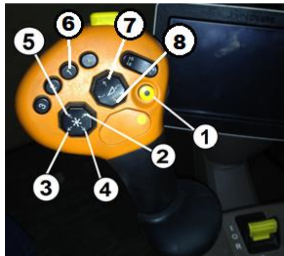
Figure 12. Merger Controls Key 1 – Merger Enable/Disable Key 2 – Belt Speed Increase Key 3 – Belt Speed Decrease Key 4 – Manual Merger Lower Key 5 – Manual Merger Raise
