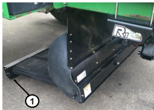
Figure 32. Down-Stop Adjustment Key 1 – Measurement Location
