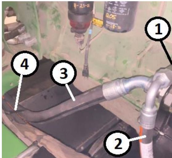
Figure 71. Pump Connections Key 1 – Pump Key 2 – Pressure (to manifold) Key 3 – Suction Key 4 – Tie Band location
