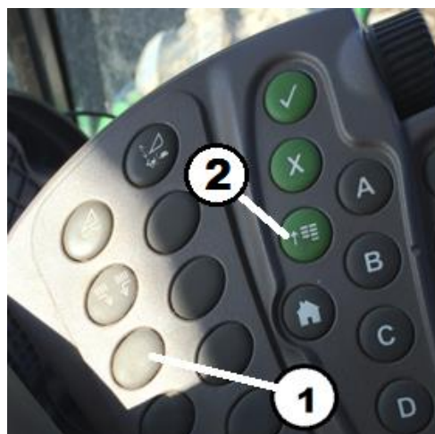
Figure 124. Armrest Buttons Key 1 – Remove Cap Key 2 – Menu Button
