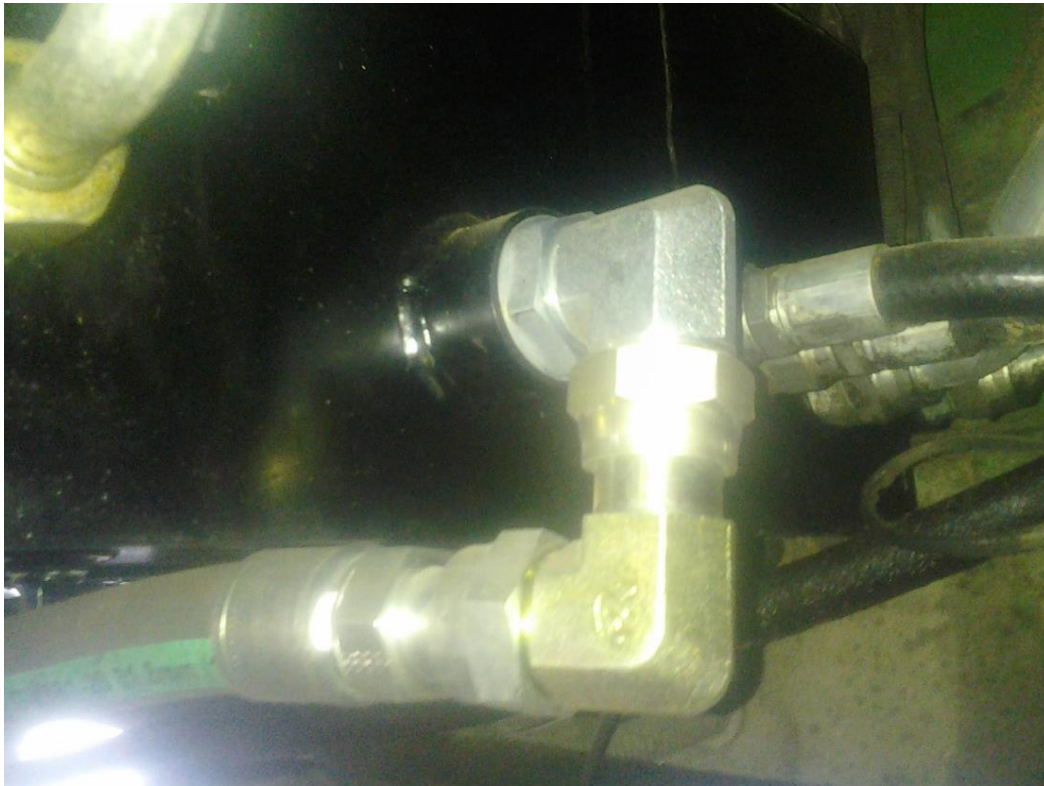
Figure 1. Suction Port Fitting Installation
