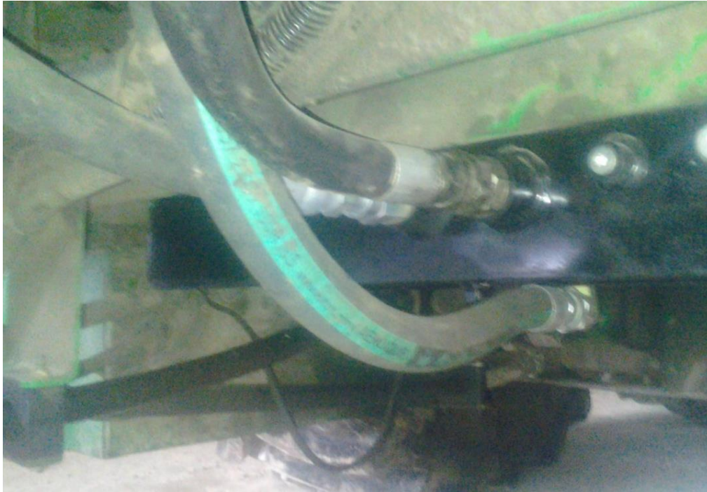
Figure 2. Suction Hose Routing
